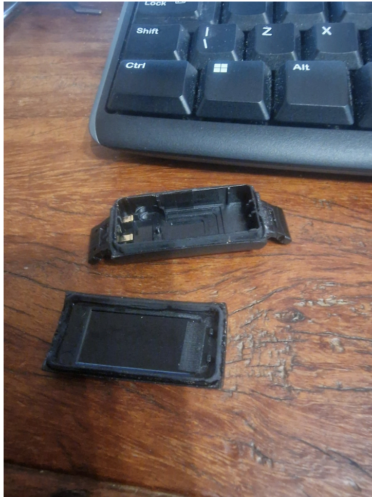
Figure 1: The housing opened: main body (top) and back plate (bottom). Both halves are intact, and the adhesive residue along both rims is visible.
