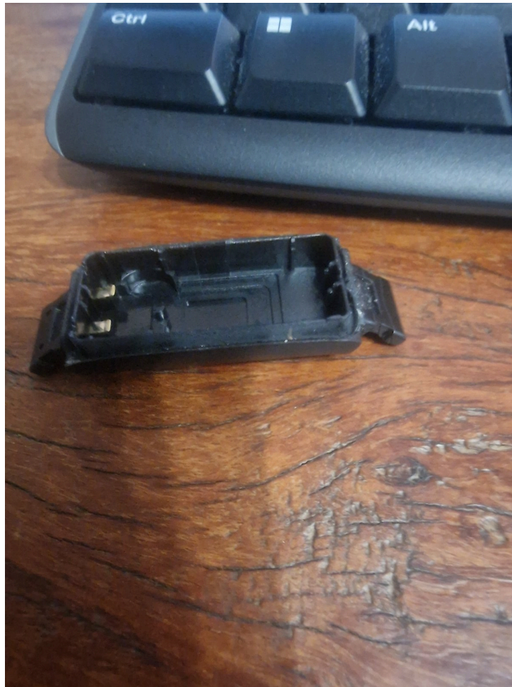
Figure 3: The empty main body. The glue channel around the rim is intact and takes a new bead of adhesive.
